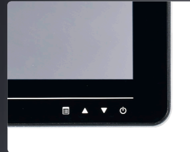
OSD Controls: Display brightness, display power on/off
