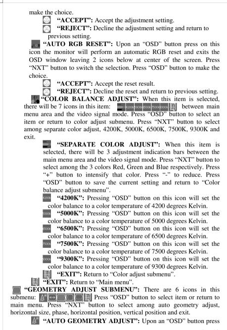
on this icon the monitor will perform an automatic geometry adjustment and exits the OSD window leaving 2 icons below at center of the screen. Press "NXT" button to switch the selection. Press "OSD" button to make the choice.
